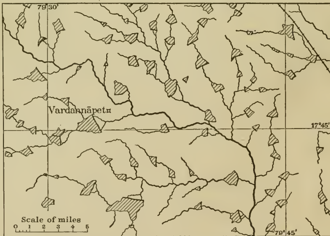
FIG. 22. Small "tanks" containing surface water impounded behind earthen dams and used for local irrigation. They occupy 1580 square miles in British India. Reduced section from the topographic map of India, scale 1 : 253,440, Sheet 56-0, 1914.
